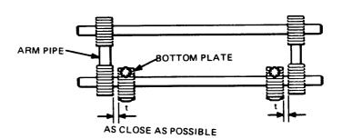
The LG60 and LG80 have the same parts, as in the diagram.
