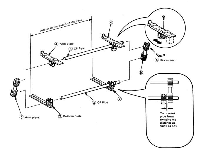
5. Slide the assembled stand onto the rails ① in step 1. Then, using the two included hex bolt ⑧, fasten the stand to the rails ① so it does not move.
