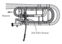
**4.** Attach the included F-valve slide to the instrument, paying attention to the insertion direction.
