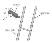
\* Only when applying a slide cream After applying a slide cream, use a water spray bottle to moisten the slide sufficiently.
