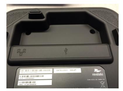
Connect one end of the Ethernet cable into the network connection port on the bottom of the unit. It's characterized by the icon displayed below. Press until it clicks into place.
