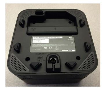
The area pictured in the figure below is where the USB and Ethernet cables are connected.
