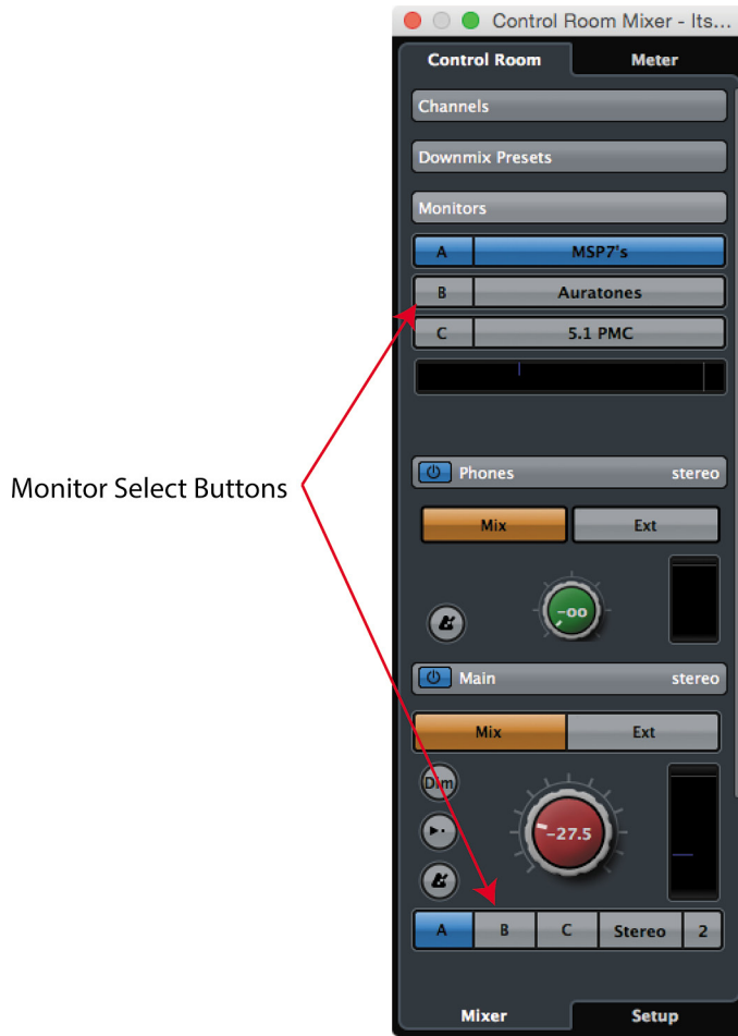
Figure 22.5 Control Room Mixer monitor selectors
