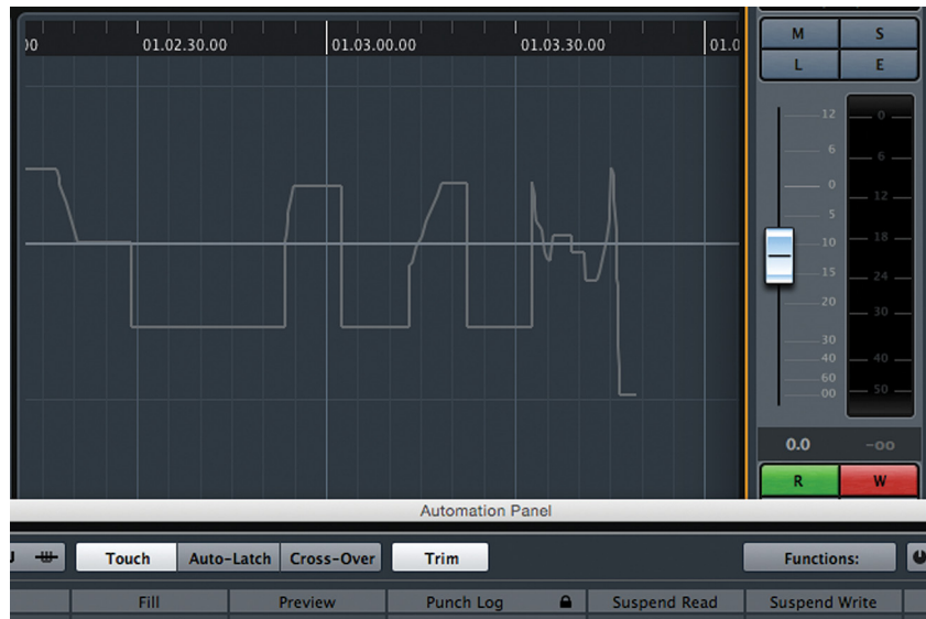
Figure 26.16 Channel in Trim mode showing trim line and fader in the middle unity position
