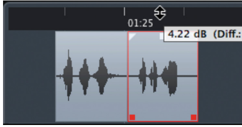
Figure 15.18 Increasing the level of the audio event using the volume handle by about 4.2 dB
