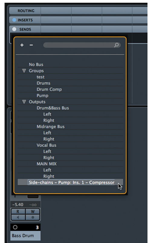
Figure 23.15 Routing the bass drum signal to the side-chain input with a send
