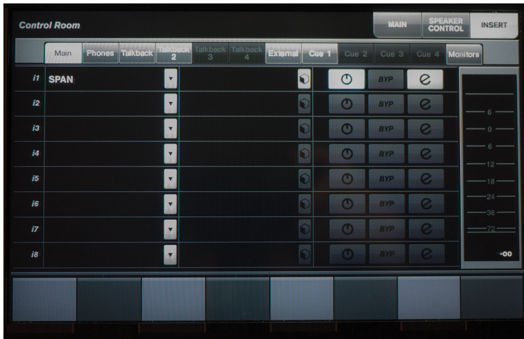
Figure 4.46 Control Room Inserts page set to Main channel
