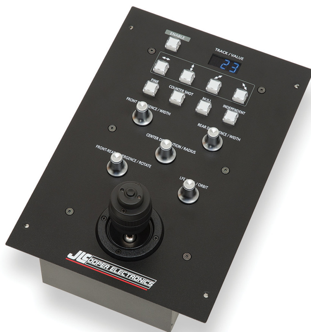
Figure 24.10 JL Cooper Nuage Joystick Panner
