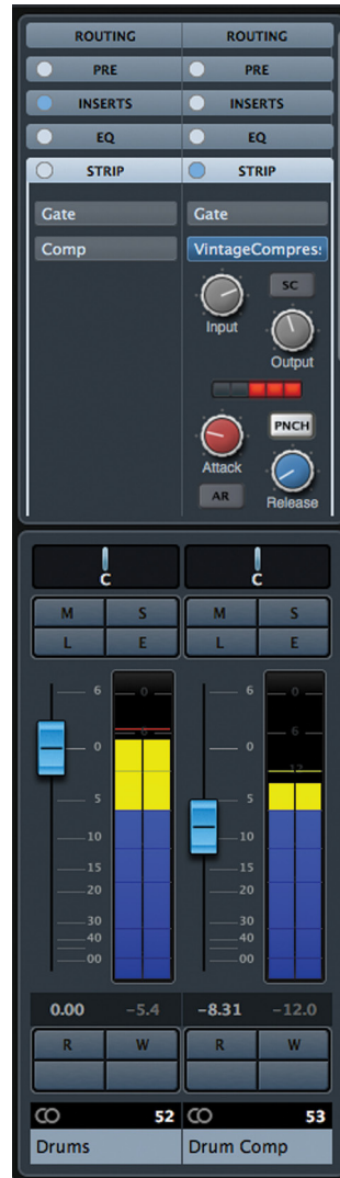
Figure 23.4 Mixing the parallel compressed track
