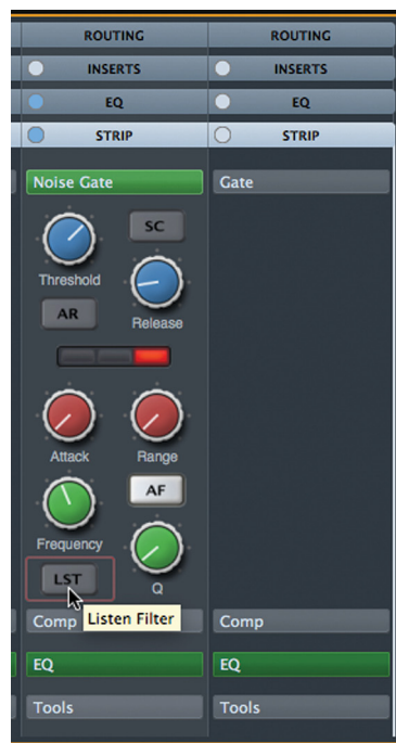
Figure 22.14 Channel Strip Gate
