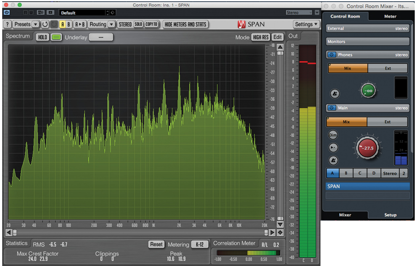
Figure 22.4 Control Room Mixer with Span meter
