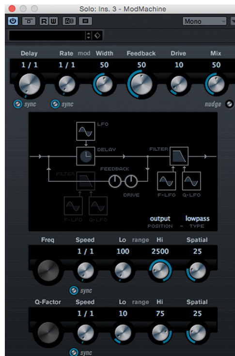
Figure 23.16 The ModMachine delay plug-in with adjustable filters and drive control on the feedback circuit
