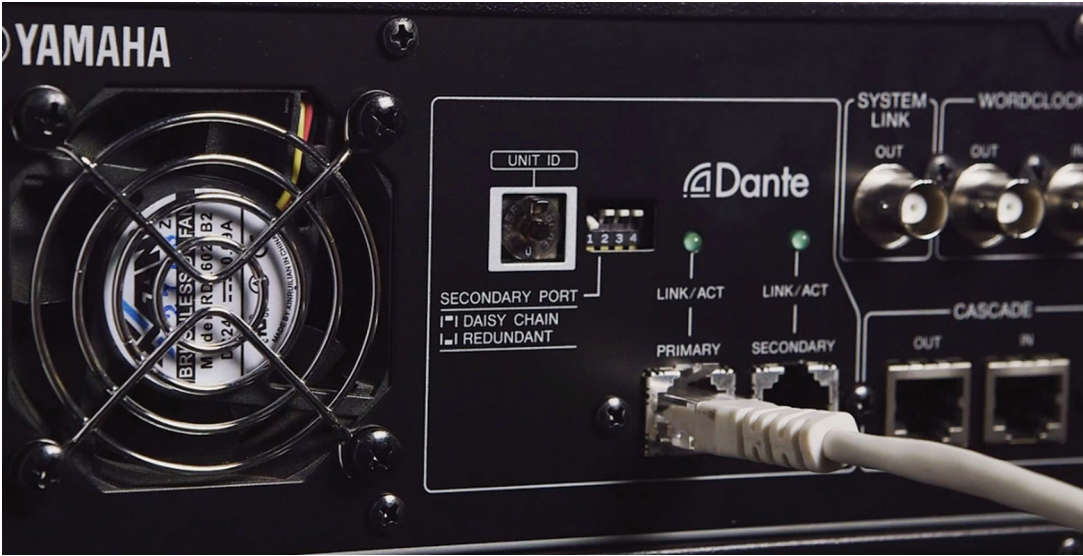
Figure 2.4 Rotary switch for device ID
